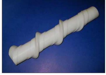
This UNITAL copolymer acetal timing screw solved the mystery of intermittent production line slowdowns because of its excellent dimensional stability due to inherent, extremely low moisture absorption compared to cast nylon.
